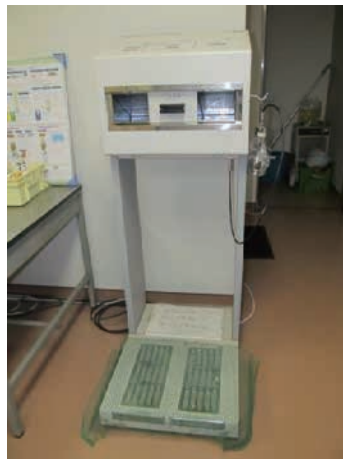
Figure 8-5 Contamination detecting equipment for hands, feet, and clothing (hand-foot-clothing contamination monitor, HFC)
