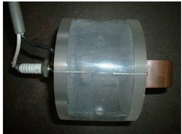
Photograph 4 Remote control discharge switch
