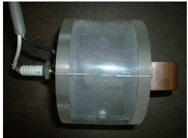
Photograph 4 Remote control discharge switch
