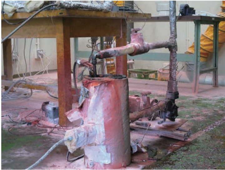
Container in which oil was heated with the electric heater (after the fire was extinguished)
