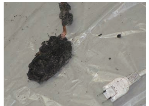
Extension cord set that was presumably the source of the fire
