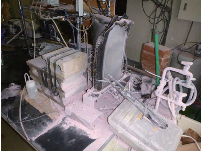
Burned test device: black container in middle is plastic water bucket
