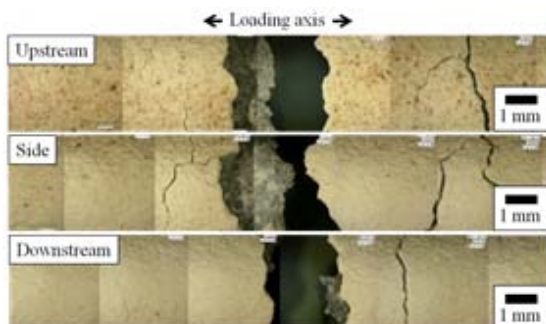
Fig. 3 Micrographs of the TBC surface after 99 thermal cycles with 170 MPa tensile loading at 700/1280°C (Mar-M247-1 TBC specimen)
