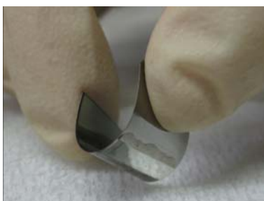
Fig.5 Photograph of bending of the FS-DMFC by human fingers.
