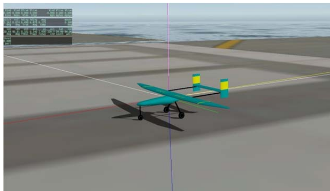
Fig. 6 Testing the AeroMas UAV model in HIL Lab
