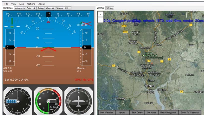
Fig.8 Ground Control System with Customized Map
