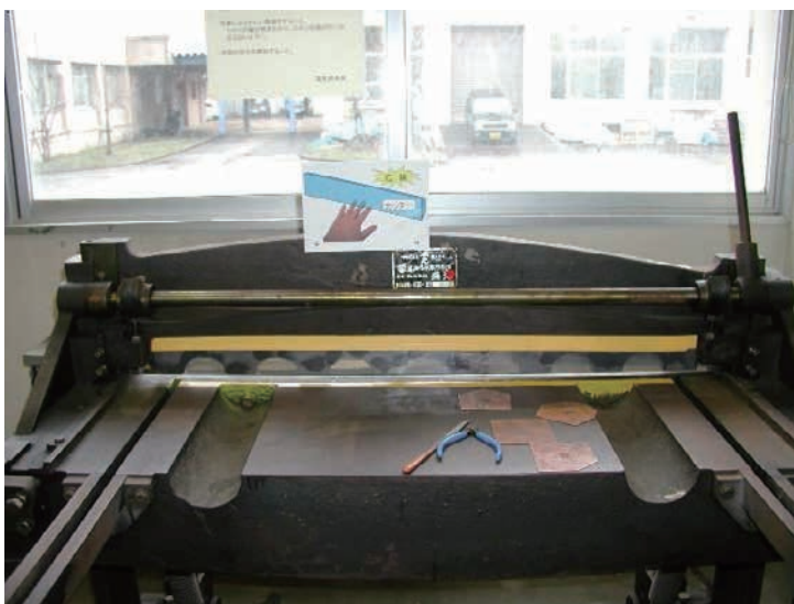
Foot-pedal-based cutting machine (after improvement)
