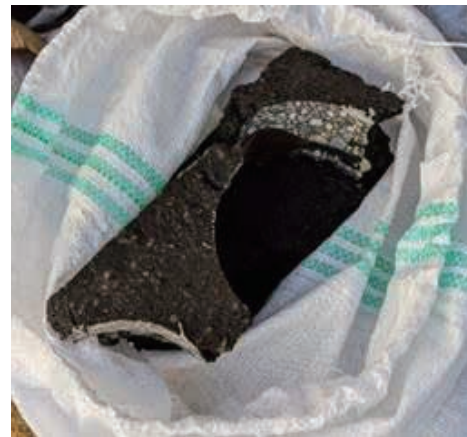
Plate-shaped asphalt concrete debris that caught fingers
