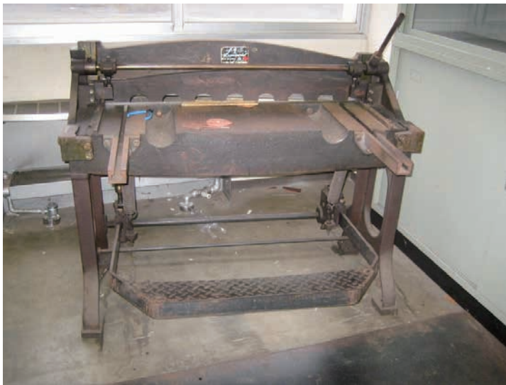
Foot-pedal-based cutting machine (before improvement)
