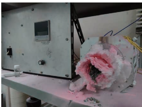
Tubular electric furnace
