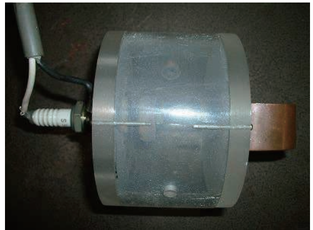
Photograph 4 Remote control discharge switch
