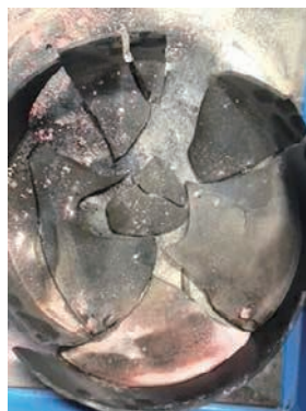
Damaged oil-receiving part
