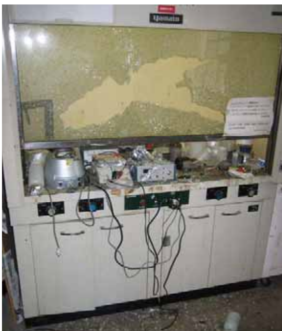
Fume hood after accident The front glass was damaged because the glass bottle burst inside the fume hood.
