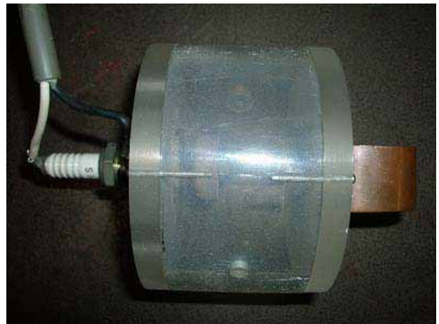
Photograph 4 Remote control discharge switch
