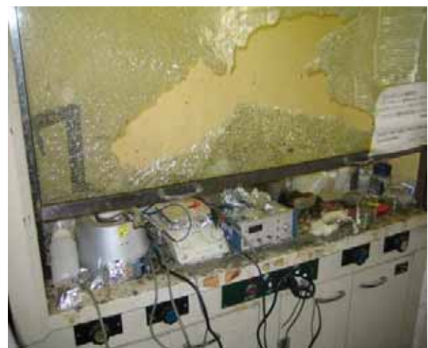
Fume hood after accident The front glass was damaged because the glass bottle burst inside the fume hood.
