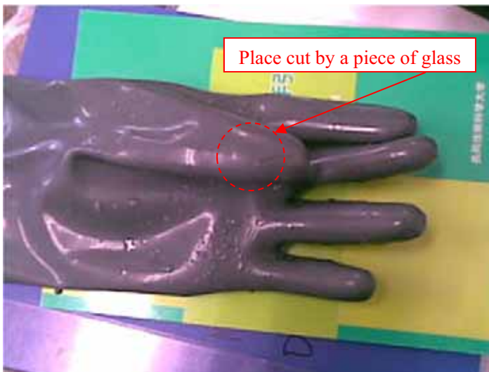
Acid-resistant gloves worn at the time of accident
