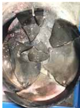
Damaged oil-receiving part
