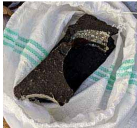
Plate-shaped asphalt concrete debris that caught fingers
