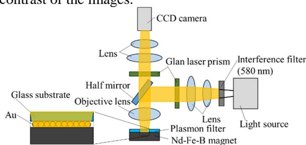
Fig. 1 Optical systems for imaging of magnetic domains.
