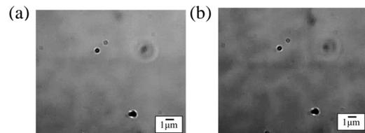
Fig. 2 Images of magnetic domains (a) without and (b) with Au plasmon filters.
