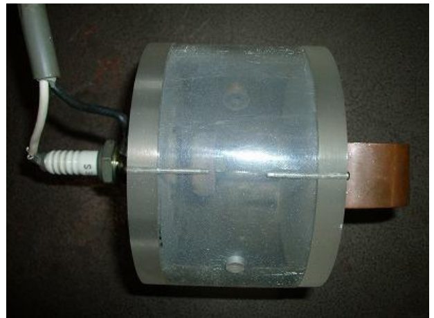
Photograph 4 Remote control discharge switch
