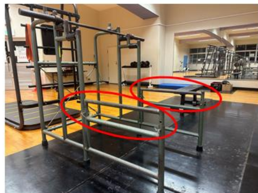
Figure 13-9. Safety Bars on the Bench Press Stand (Top) and Squat Rack (Bottom) (Highlighted by Red Circles in the Photo)
