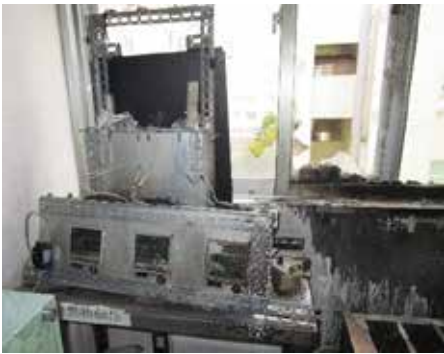
Small electric furnace that was in operation at the time of the fire
