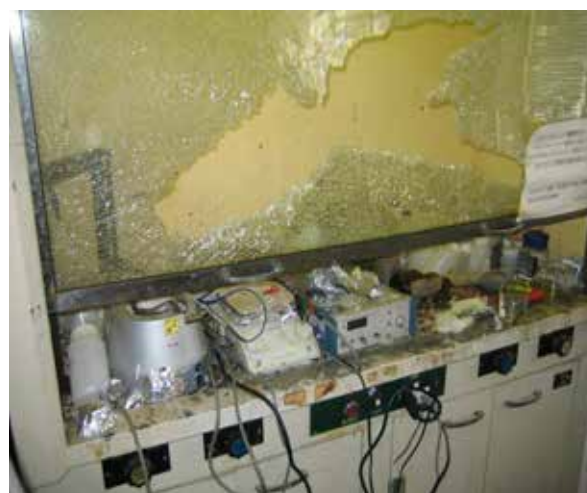
Fume hood after accident The front glass was damaged because the glass bottle burst inside the fume hood.
