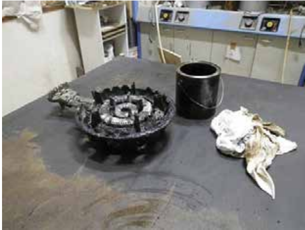
Asphalt container, stove, and waste cloth
