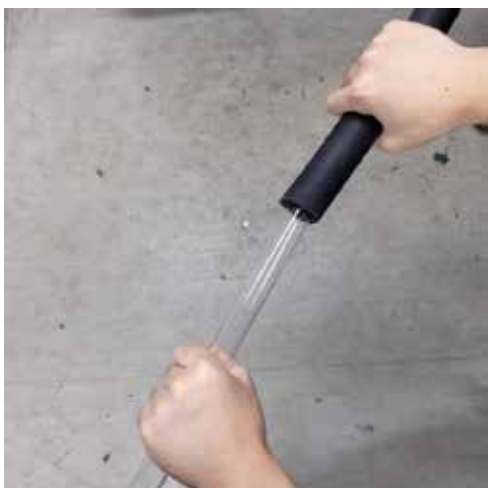
Connecting quartz tube to hose
