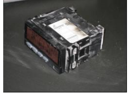
Partially burnt voltage indicator
