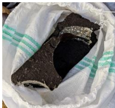
Plate-shaped asphalt concrete debris that caught fingers
