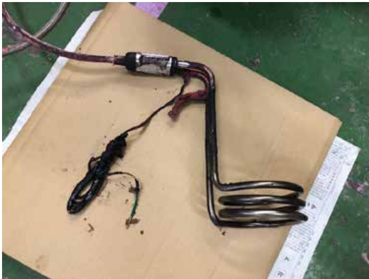
Electric heater that was installed in the container that contained oil
