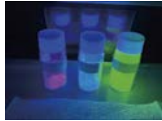
The luminescence of phosphor materials fabricated in our laboratory
