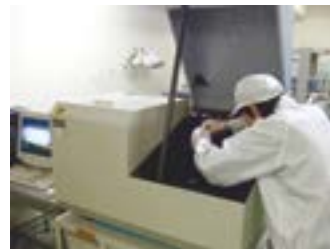
Measurement of liquid crystal panel using spectroscopic ellipsometer
