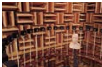
A dummy head and speakers set in the anechoic room
