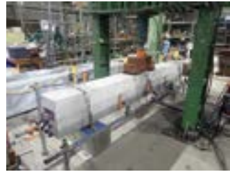
Loading Test of Prestressed Concrete Beam
