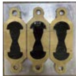
Force ductility test: (a) asphalt binder specimens; (b) specimen being pulled apart; (c) fractured specimen
