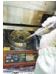
Preparation of magnetic garnet thin films by the metal-organic decomposition (MOD) method.
