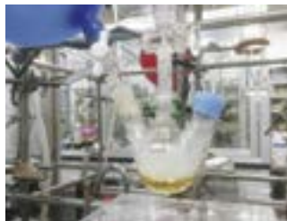
Typical apparatus of a reductive coupling reaction by magnesium metal
