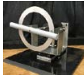
A wind turbine with circular cylinder blades driven by longitudinal vortices.
